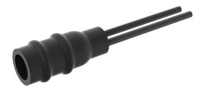
KD503 connectors have been industry requirement for over 30 years. They are designed for a fast-and-easy watertight connection between the secondary cable and the series isolating transformer. This connector is silicon and used with two single core wires. Connector is fast to install, approx. 1min. KD 503 connectors are FAA certified.
