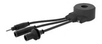
An Airfield Ground Lighting (AGL) transformer, also named isolation transformer, is typically installed in series circuits in airport approach line, runway, taxiway and other airport lighting systems to provide right amount of current to the low voltage lights respectively along the circuit and to ensure main circuit continuity in case of light failure.
